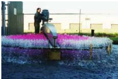
Johnson Screens has patented an advanced collector distributor system design that allows for fractal control of fluid flow in a media. This flow is demonstrated by the even distribution of the dye through the water.
