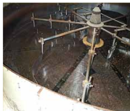
Johnson's screens can be used in numerous applications, such as this lauder tub, used to separate grains from the wort in the brewing process.
